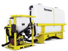
**Vermeer drilling fluid systems**provide the horizontal directional drill with quality mud mixing in a minimum amount of time. Smaller systems are self-contained on a mounting skid. Larger systems are available preassembled on mounting platforms to provide drilling operations with greater versatility.
