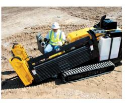
**Rod-carrying capacity** An onboard rod-carrying capacity of 300' (91.4 m).
