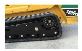
DON'T WEAR IT OUT. A high-mounted track sprocket eliminates wear caused by ground contact.
