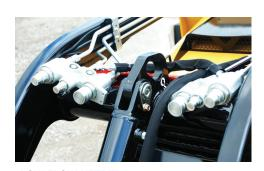
LOW FLOW NEEDED. An optional dual hydraulic auxiliary adds a low-flow option to the hydraulic circuit for use with dual-function attachments.
