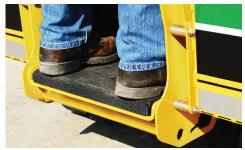
ABOVE THE FRAY. A dedicated, spring-cushioned platform keeps the operator out of the mud. The integrated operator presence system suspends ground drive and powered boom/bucket motion when the operator steps off the platform.
